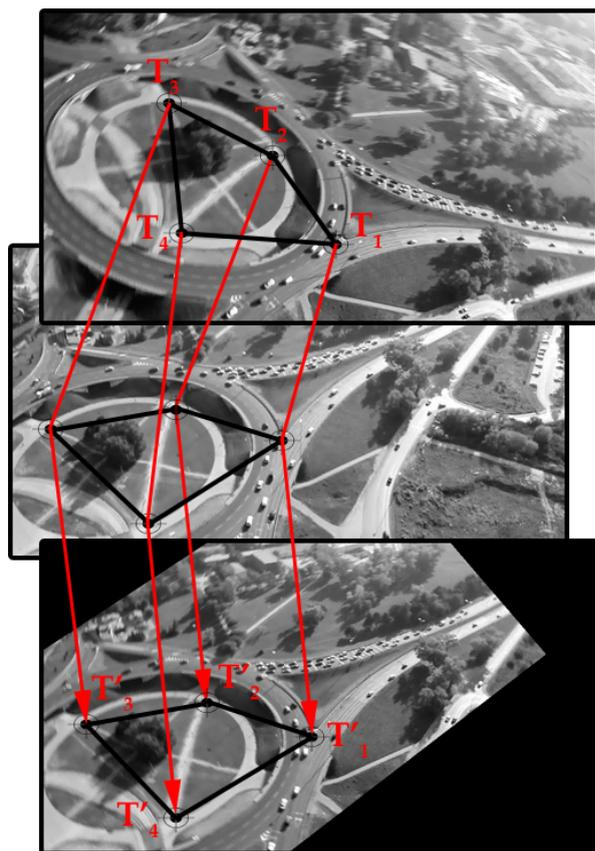
Fig. 2. Stabilization of video acquired from hovering aircraft. The figure shows the current frame (top), the reference frame (middle), and the transformed current frame (bottom). Points  $T_i$  in the current frame are transformed to the points  $T'_i$  by the homography between the current frame and the reference frame.
